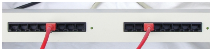
16-port RDA in 1U 19" rack. Configurable as either 2 x 8-port RDA's or as a 1 x 15-way system (using 1 port as loop-thru)
